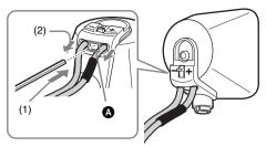
When the lever is down, the speaker cords are locked.
